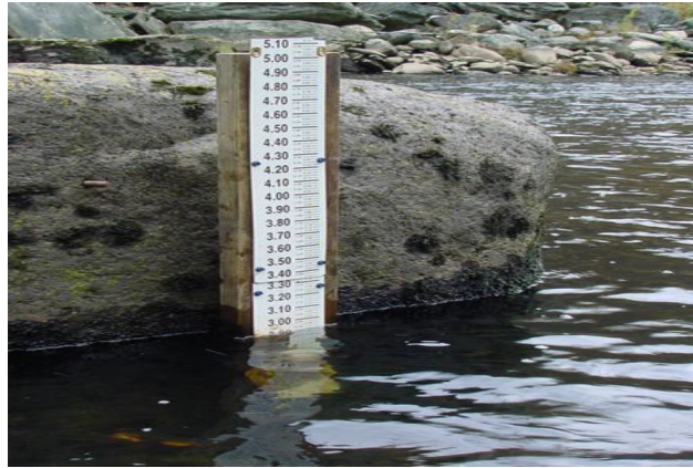
This staff gauge reads a stage value of 2.92 feet (Parker 2004).
