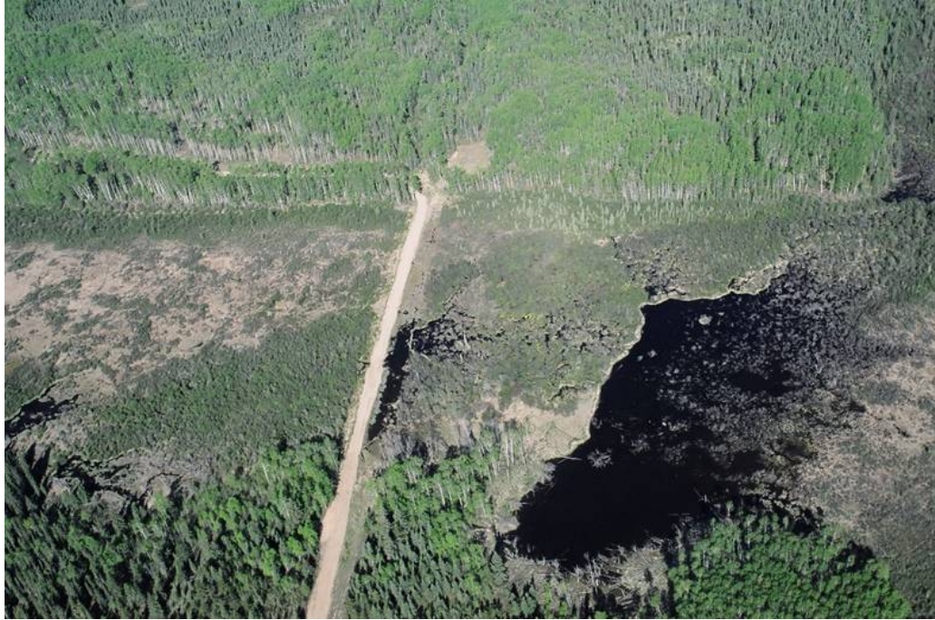
Figure 3.1 Example of Potential Effects of a Road Running across a Wetland Perpendicular to Water Flow, Causing the Water Table to Increase on the Right and Decrease on the Left
