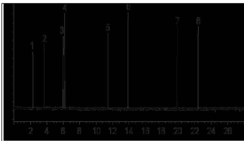
**Figure 2.** Chromatogram of 200  $\mu\text{g}$  S/L Standard Containing (1) Total Sulfide; (2) MeSH; (3) DMS; (4)  $\text{CS}_2$  (resolution check compound); (5) Thiophene (internal standard); (6) DMDS; (7) DMTS; (8) Thioanisole (internal standard)
