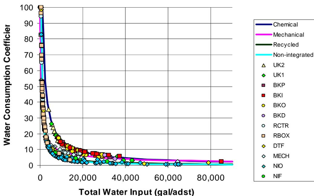
**Figure 4.6** Water Consumption for U.S. Mills as a Function of Total Water Input, with Individual Contributions from Secondary Waste Treatment Type [See Appendix A for category definitions.]
