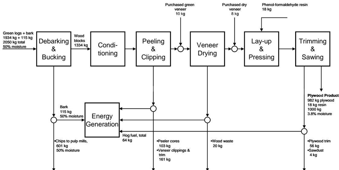
**Figure C.5** Southeastern Softwood Plywood Mill Weighted Average from 5 Facilities, wood(dry) mass balance [wood mass balance extracted from Wilson and Sakimoto 2005]
