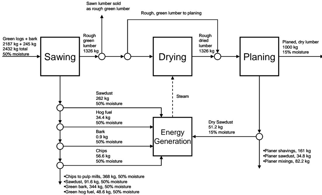
**Figure C.3** Hardwood Lumber Mill Weighted Average from 20 Facilities in 20 States, wood(dry) mass balance [wood mass balance extracted from Bergman and Bowe 2008]
