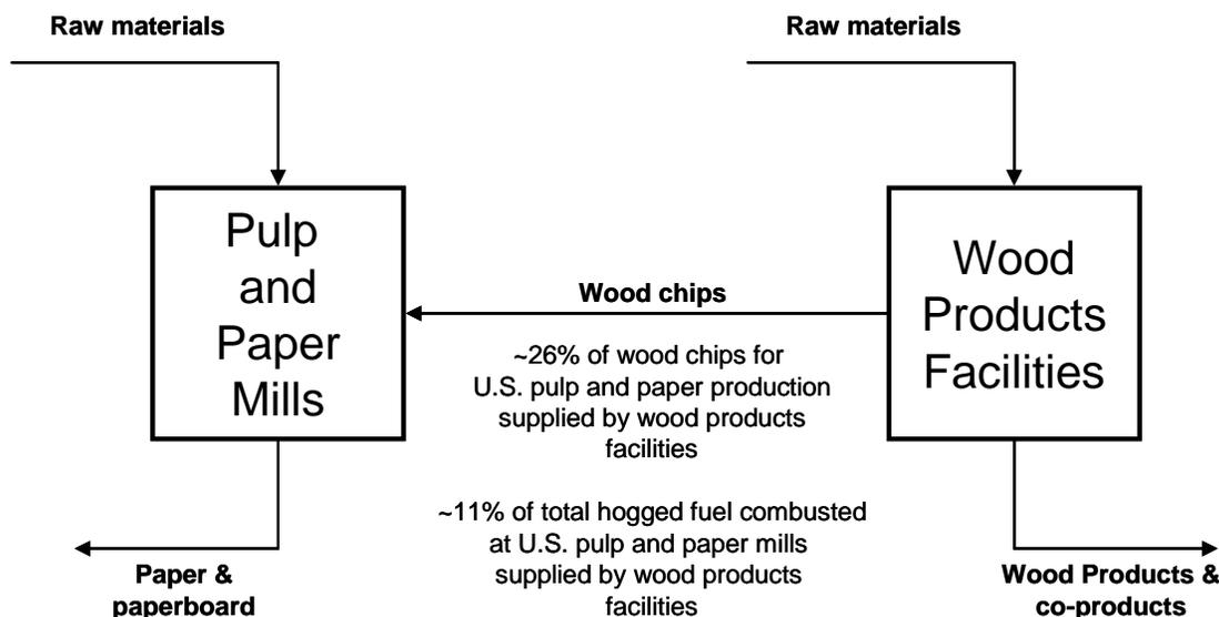
**Figure 4.8** Interplay Between U.S. Wood Products Industry and U.S. Pulp and Paper Industry
