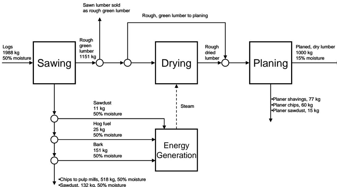
Figure C.1 Pacific Northwest Softwood Lumber Mill Using Douglas Fir and Hemlock [wood mass balance extracted from Milota 2004; Milota et al. 2004, 2005]
